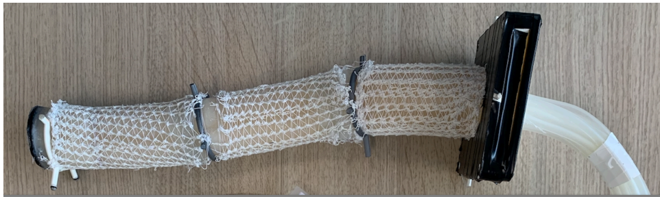
Figure 1: A pneumatic soft robot consisting of three segments. Each segment can bend in any direction by inflating its four air chambers.
